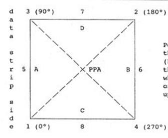
Positions of all points are referenced to the principal point of autocollimation (PPA) as origin. The diagram indicates the orientation of the reference points when the camera is viewed from the back, or a contact positive with the emulsion up. The data strip is to the left.
