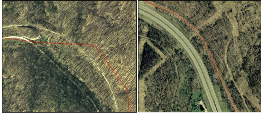
Figure 10. Scale issues, North Bend Rail Trail, original data (left), repaired data (right)
