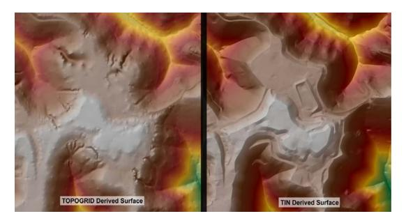
Figure 2. Comparison between TOPOGRID and TIN derived surfaces.
